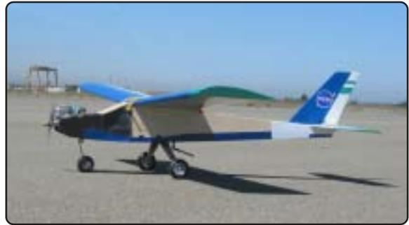
autopilot that provides state information. Software on the PC 104 is used to control of the aircraft via a two-way air to ground control link and a servo control switch. The aircraft is flown up to altitude using conventional RC control then "handed over" to the computer-based operator on the ground.
