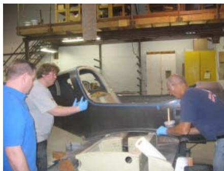
Attaching the fuselage to the center wing.
