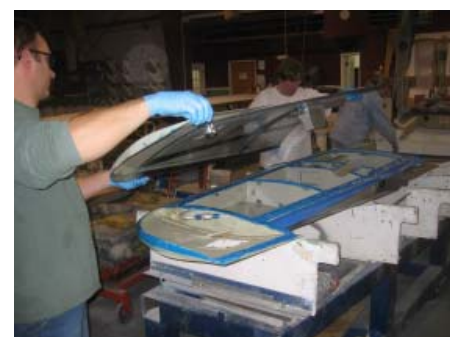
Bonding a Legacy wing at the Lancair factory.
