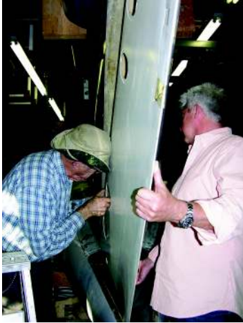
Rusty and Mike fitting the rudder
